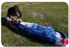
**Step 8**. Lay the Folding Pillow in place and make the fold of the LE around it. Use 3 folds.
